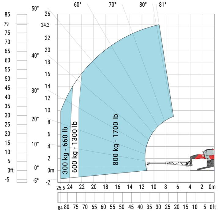
Machine on lowered stabilisers with winch 6000 kg (Metric)
