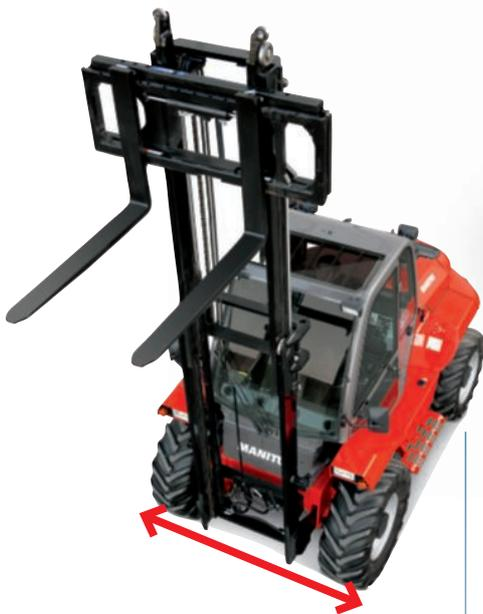
Its **width** ensures the fork-lift truck has better stability for extra safety for lateral loading.
